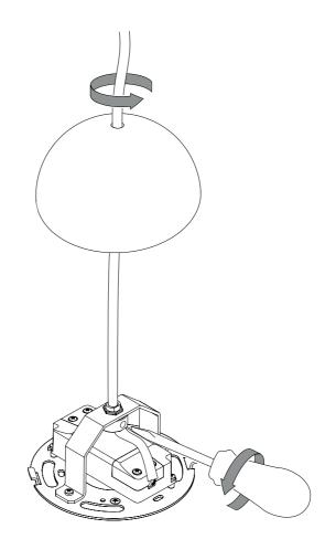
Loosen the two screws holding the terminal cover and remove the terminal cover.
