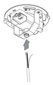
After inserting the cable through the cable grip, as shown in the previous step, locate the fibre support cable and feed it through the small hole next to the exit hole on the cable grip (1). Once the fibre support cable has exited the other side, as shown below, the smaller fixed screw on the side of the cable grip can be fastened with the provided hex key, securing the fibre support cable in place (2).
