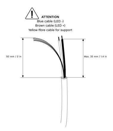
It is advised that any wire exposed with just a single basic layer of insulation is covered with the protective heat shrink provided. (Two sleeves for the basic insulated wire and one sleeve for covering the opening of the source cable). A heat gun can be used to shrink and fix this protective insulation in place (2). The double insulated mains power cable that connects to the LED driver should have a diameter between 2 x 0.75 mm<sup>2</sup> - 2 x 1.5 mm<sup>2</sup>.
