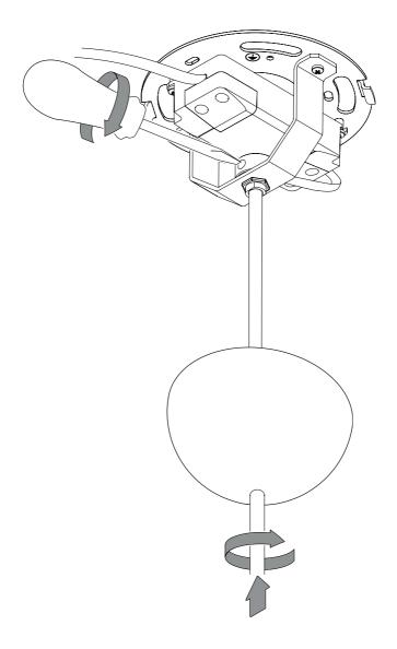
Due to the handmade manufacturing of the glass shade some shades will have a slight difference in the distribution of weight, which can cause them to tilt slightly. If this happens, you should reposition the three supportive legs inside the shade, adjusting them until the shade is level.
