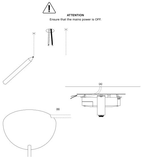
Drill holes and insert wall plugs. Ensure you use the correct type of drill and anchor for the type of ceiling you are drilling into.
