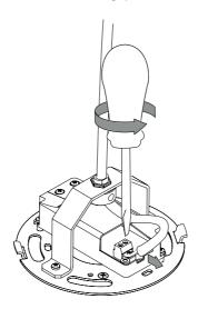
Use a pencil to mark fixing holes in the ceiling where the pendant is to be mounted. If there is a junction box in the ceiling, then the steel bracket has slots which can be used in conjunction with standard European and US junction boxes. If relevant, the input mains cable can be inserted through the centre hole in the steel bracket and passed beneath the LED driver. The input mains cable can also be inserted through the mousehole on the side of the plastic ceiling canopy if needed.
