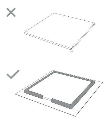
Insert the leg profiles in each end of the tabletop frame.
